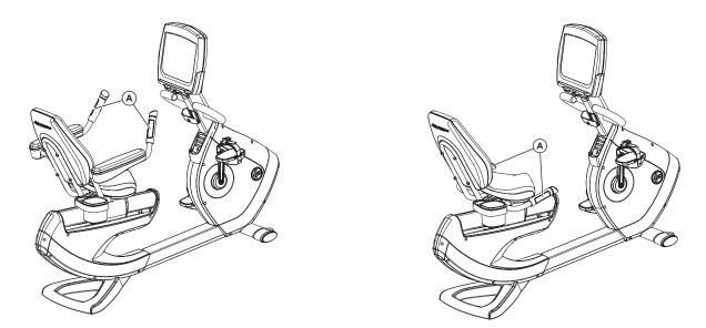
Grasp the sensors that are located on either the armrests or the side handlebars of the Recumbent Lifecycle Exercise Bike.
